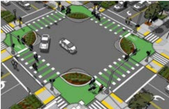
A **protected intersection** physically separates bicyclists and pedestrians from vehicle traffic at an intersection to reduce areas of conflict with vehicles. Protected intersections have separated crossing facilities to reduce crossing distance, enhance pedestrian and bicyclist visibility to vehicles, and encourage lower speeds.
